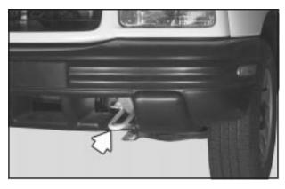
Your vehicle is equipped with recovery hooks. The hooks are provided at the front and rear of your vehicle. You may need to use them if you are stuck off-road and need to be pulled to some place where you can continue driving.
